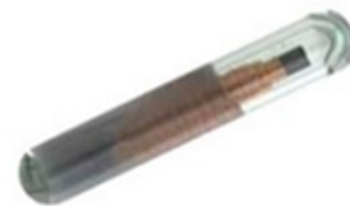
Figure 36. A PIT is a microchip included in a small sterile glass capsule injectable with a syringe.
