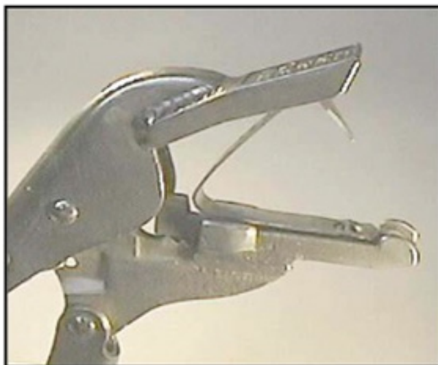
Figure 34. Position of the Monel tag ready to be stapled in two applicator models.
