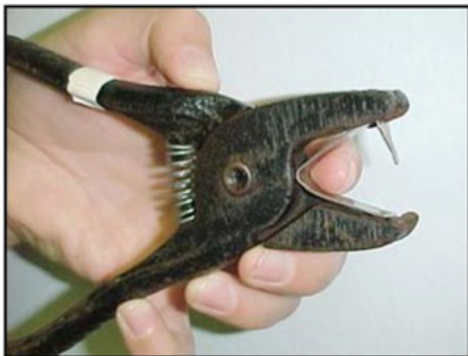
Figure 34. Position of the Monel tag ready to be stapled in two applicator models.
